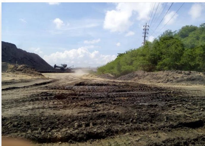
Figure 11. Wet road system that prevents air pollution in the roadways
